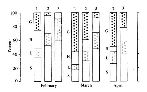
The plants have been divided into four components, viz. stems (S), leaves (L), grain (G), and non-grain (H) components of the ear. Four general features are apparent:
