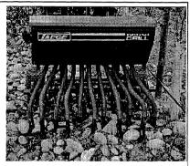
Fig. 4. Mini drill direct seeding into stoney ground between grape vines.
