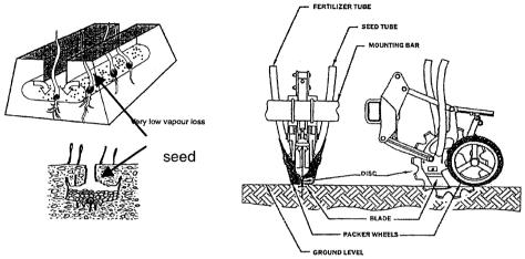
Fig. 1. "Inverted-T" slot shape (after Carter, 1994; Baker *et al.*, 1996).
