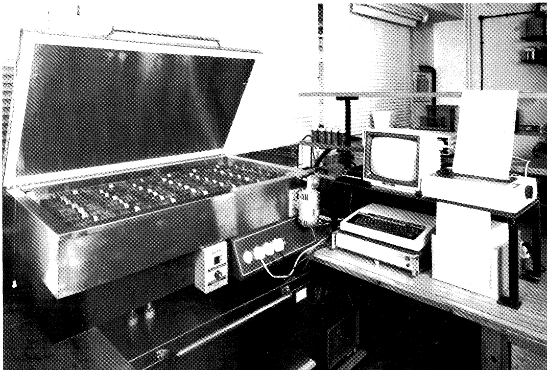
Figure 2. Computer-controlled micromalting apparatus.
